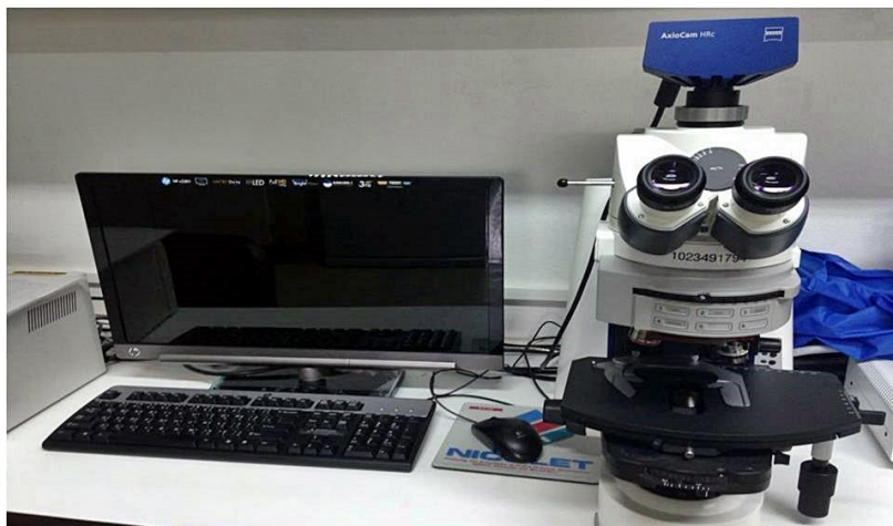
Figure 1: Photomicroscope AxioVision 40 attached to computer with AxioVision software version 4.6.3.0
