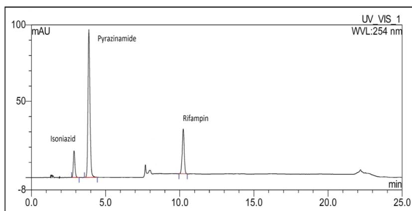
**Figure 2** HPLC chromatogram of 33 µg/mL INH, 165 µg/mL PZA, and 66 µg/mL RIF at 254 nm by using acetonitrile (A) : 3% acetonitrile in 10 mM KH<sub>2</sub>PO<sub>4</sub> pH 6.8 (B) gradient a mobile phase
