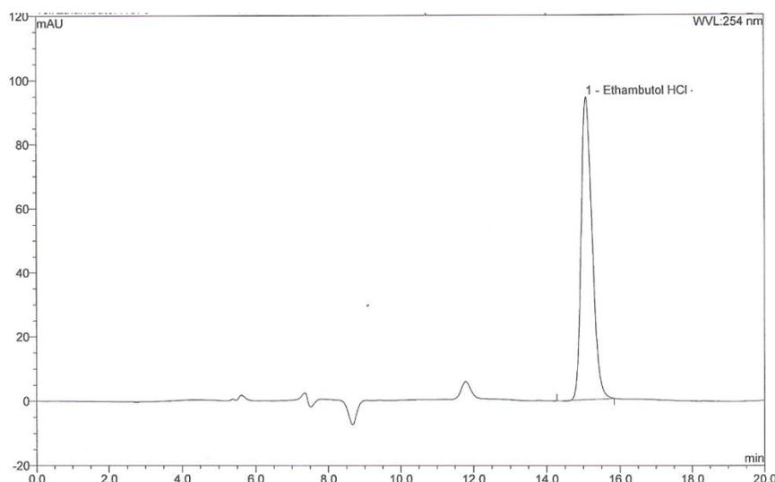
**Figure 3** HPLC chromatogram of 100  $\mu\text{g/mL}$  ethambutol at 254 nm using tetrahydrofuran: a mixture of 2 mM of copper sulfate ( $\text{CuSO}_4 \cdot 5\text{H}_2\text{O}$ ) and 3 g/L sodium hexanesulfonate in distilled water pH of 4.5 (25: 75) as a mobile phase
