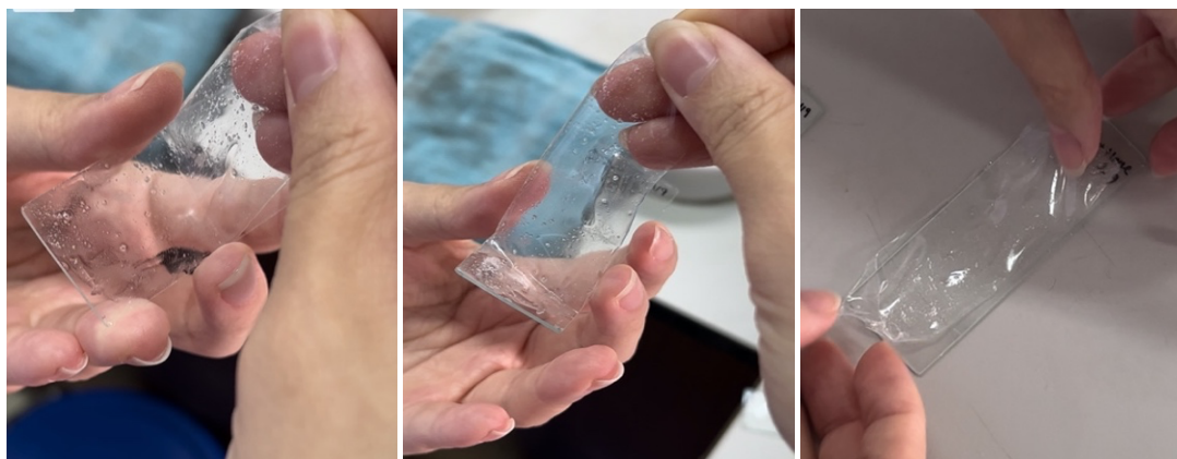
Figure 1 The dried film can be entirely removed from the the glass slide without tearing
