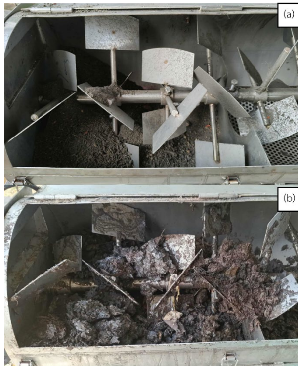
Figure 5 Physical characteristics of the composted food waste material after 7 days under in-vessel composting machine (a) and conventional composting without machine operation (b).
