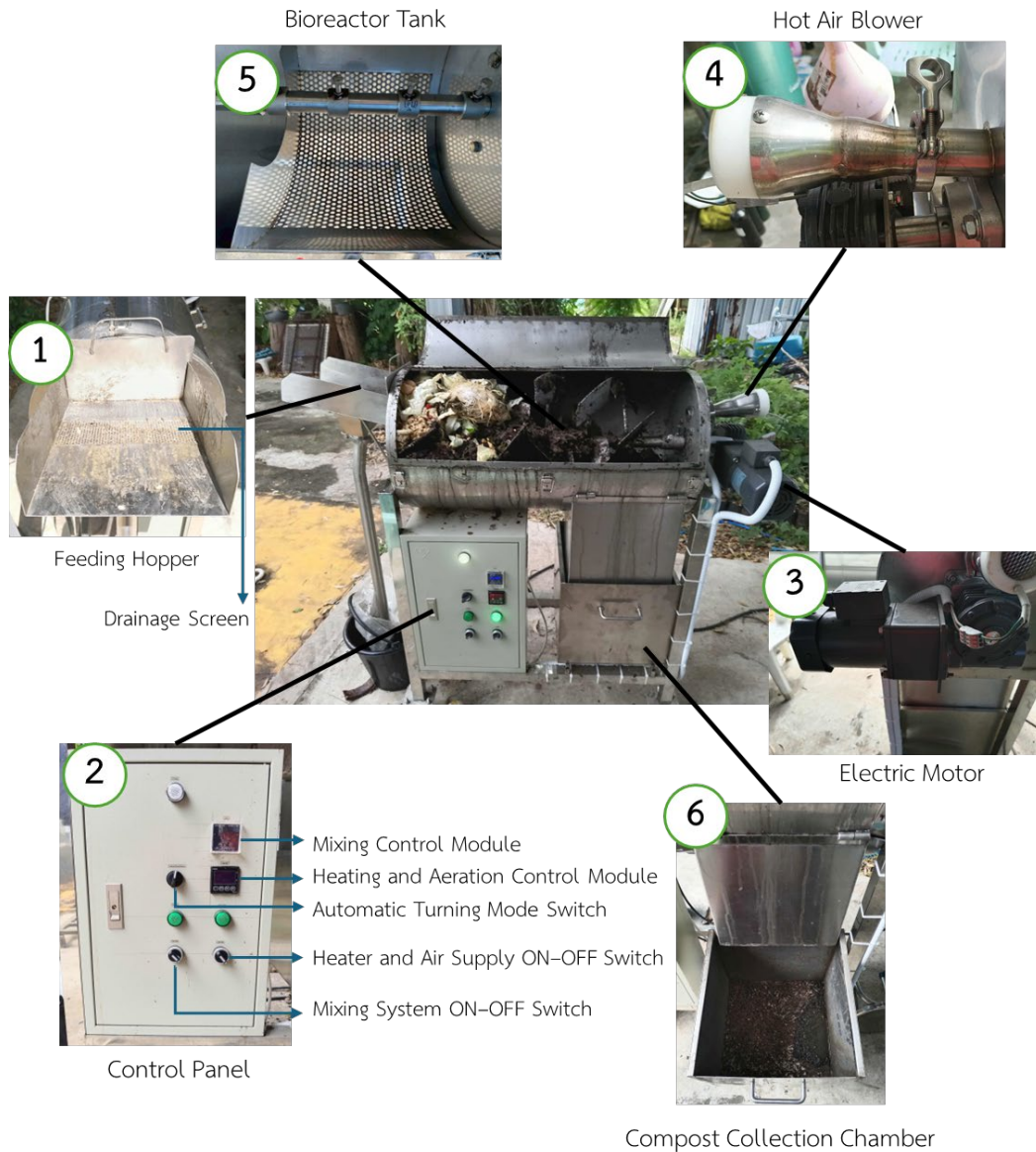
Figure 1 In-vessel bioreactor composting machine and its major components: (1) feeding hopper, (2) control panel, (3) electric motor, (4) hot air blower, (5) bioreactor tank, and (6) compost collection chamber.
