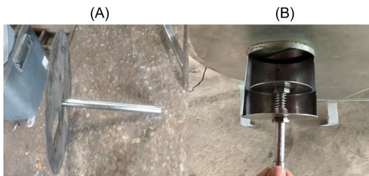
Figure 5 (A) Blade plate and (B) Axle shaft of vegetable shredder built
