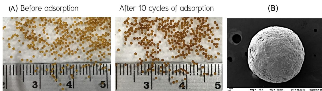
Figure 9 The CS-1.5hH hydrogel beads (A) digital photographs, scale in cm unit and (B) SEM micrograph after 10 cycles of adsorption-desorption
