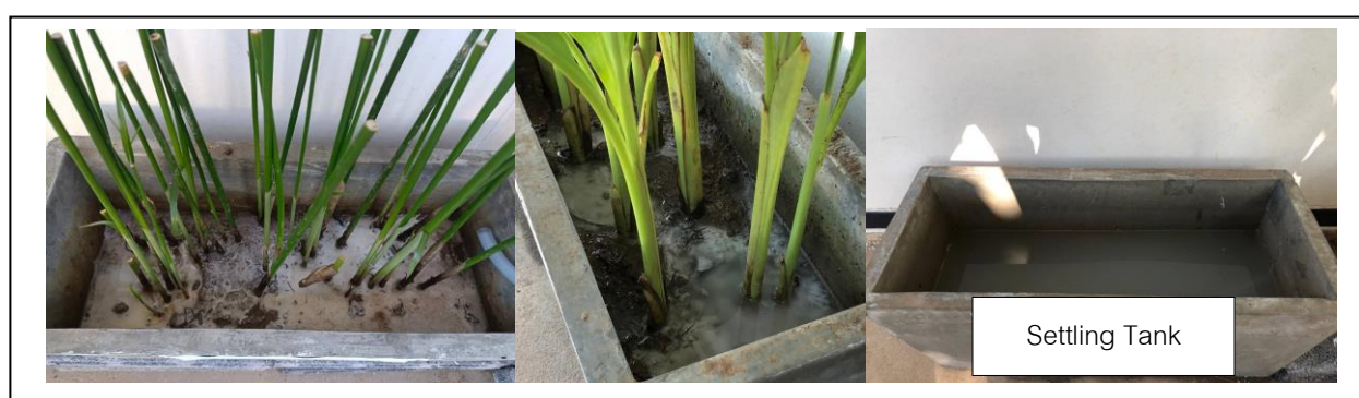
Figure 7 Suspended solid sedimentation caused by starch accumulates on the soil surface in wastewater treatment ponds
