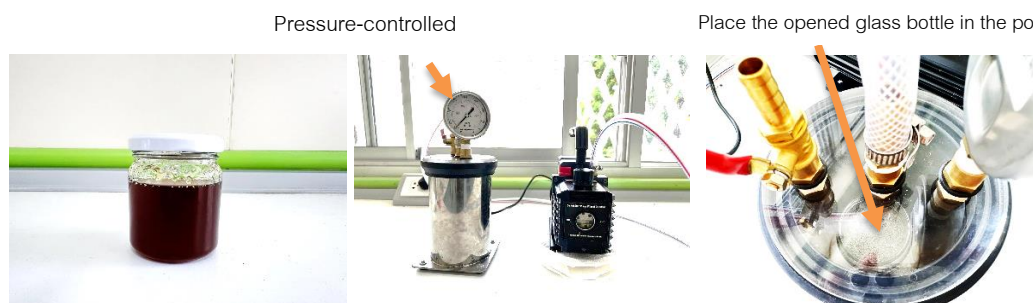
Figure 1 Application of a vacuum dehydrator for moisture removal in stingless bee honey
