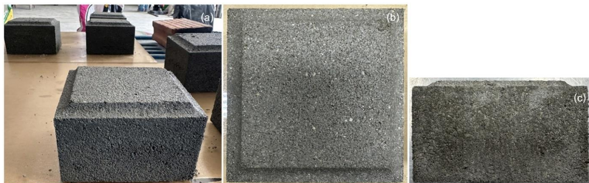
Figure 10 Dual-layer paving blocks fabricated via hand compaction: (a) perspective view, (b) top view, and (c) side view
