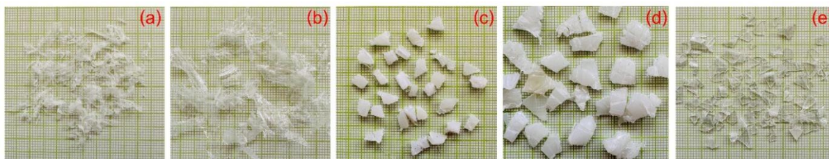
Figure 4 Plastic samples after shredding: (a) LDPE fragments smaller than 5 mm, (b) LDPE fragments between 5 - 15 mm, (c) HDPE fragments smaller than 5 mm, (d) HDPE fragments between 5 - 15 mm, and (e) PET fragments smaller than 5 mm
