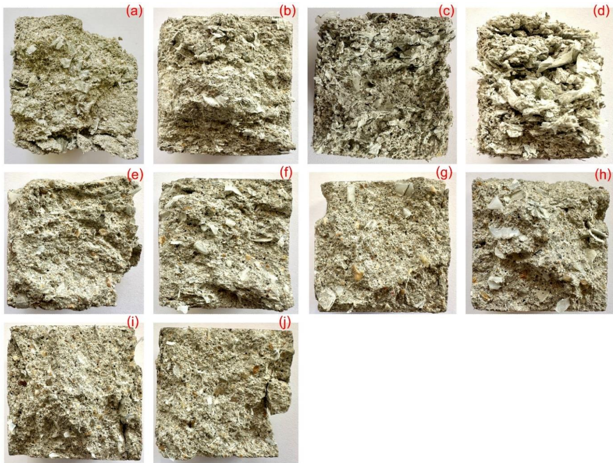
Figure 7 Internal views of mortar specimens incorporating plastic waste: LDPE fragments at (a) < 5 mm, 0.05%, (b) < 5 mm, 0.10%, (c) 5 – 15 mm, 0.05%, and (d) 5 – 15 mm, 0.10%; HDPE fragments at (e) < 5 mm, 0.05%, (f) < 5 mm, 0.10%, (g) 5 – 15 mm, 0.05%, and (h) 5 – 15 mm, 0.10%; and PET fragments at (i) < 5 mm, 0.05%, (j) < 5 mm, 0.10%
